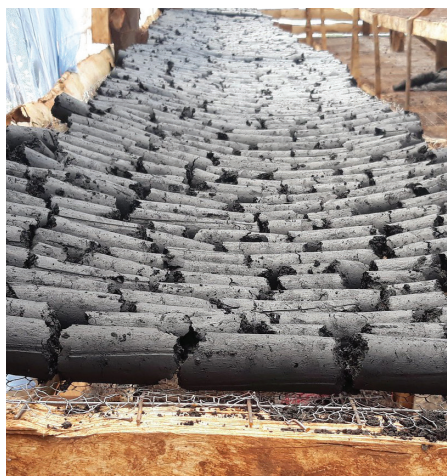
Biomass briquettes are made from sawdust, corn husks and other waste materials.
